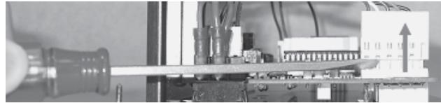
**Figure 4: Depicting the Proper Way to Remove Wire Harness Connectors Using a Flathead Screwdriver**
